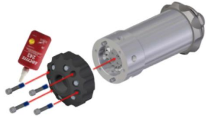
Figure 3 Maintaining the drive nozzle
